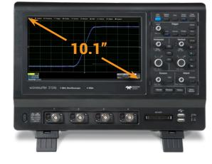
Digital Voltmeter Logic Analysis with 16 Mixed Signal Capabilities **20 Mpts** Powerful Triggering Superior Measurement Tools History Mode Anomaly Detection WaveScan LabNotebook Waveform Generator Multi-Instrument Capabilities Powerful, Protocol Analysis with Serial Trigger and Decode Pass/Fail Mask Testing Advanced Math The WaveSurfer 3000z has a 10.1" capacitive touch display, the longest memory, and the deepest toolbox – all at an affordable price.
