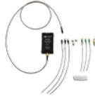
Specifically designed to probe a low impedance power/voltage rail. The RP4030 has 30V built-in offset adjust, low attenuation (noise), and high DC input impedance with 4 GHz of bandwidth and a wide assortment of tips and leads, including solder-in and U.FL receptacle connections.
