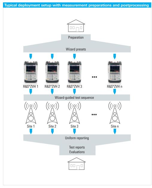
Test sequences can be predefined on a central PC and transferred to all R&S°ZVH analyzers that will be used on a project. On-site, the R&S°ZVH wizard guides the user step-by-step through the predefined test sequence. All measurement results are stored in a single file which can easily and centrally be converted to a uniform, well-structured test report using the R&S°ZVHView software.
