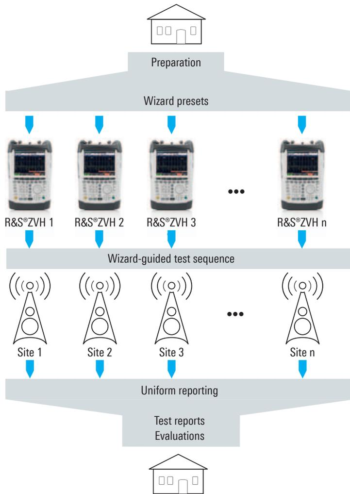
Test sequences can be predefined on a central PC and transferred to all R&S ZVH analyzers that will be used on a project. On-site, the R&S ZVH wizard guides the user step-by-step through the predefined test sequence. All measurement results are stored in a single file which can easily and centrally be converted to a uniform, well-structured test report using the R&S ZVHView software.
