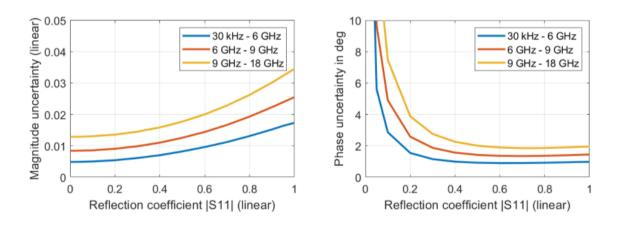
Reflection uncertainty, measurement bandwidth of 10 Hz, nominal source power of -10 dBm and a coverage factor of k = 1 (67 % confidence interval)
