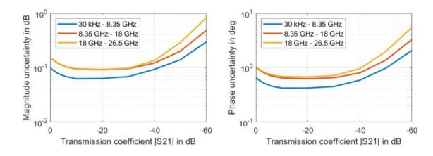
Transmission uncertainty, measurement bandwidth of 100 Hz, nominal source power of -10 dBm and a coverage factor of k = 1 (67 % confidence interval)
