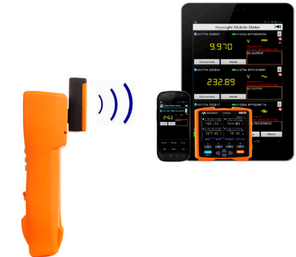
U1240C series is compatible with Keysight Remote Link solution to safely measure, view and log test measurements.
