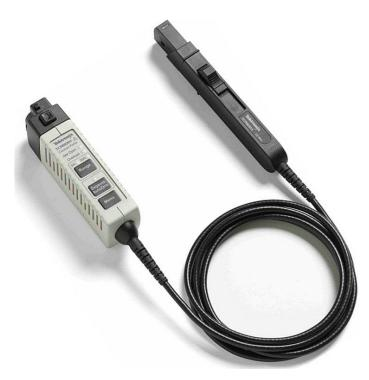
TCP0030A is a high-performance, easy-to-use AC/DC current probe designed for use and direct connection to oscilloscopes with the TekVPI™ probe interface. This AC/DC current measurement probe provides greater than 120 MHz of bandwidth with selectable 5 A and 30 A measurement ranges. It also provides exceptional low-current measurement capability and accuracy to current levels as low as 1 mA, important for meeting today's challenging current measurement needs.
