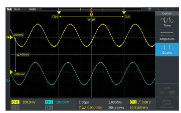
The cursor readouts are presented on the waveform display. Cursors can be used to measure time and amplitude.
