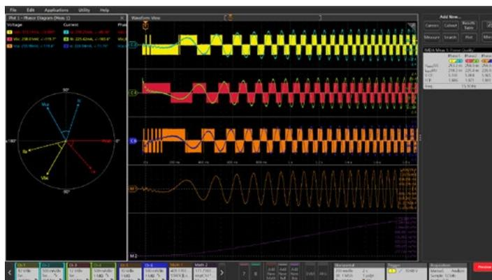
Automate common measurements such as true power, apparent power, reactive power, power factor and many more.
