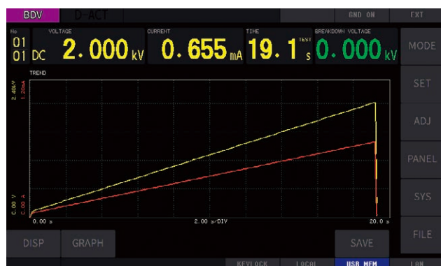
Example of continuous voltage rise test
