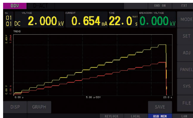
Example of stepped voltage rise testing
