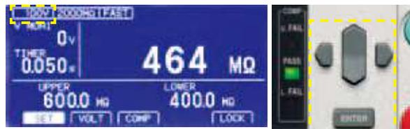
The test voltage can be changed simply by pressing the keys and verified on the screen.
