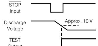
[FAST]: The signal returns to high at about the same time as the test is completed.
