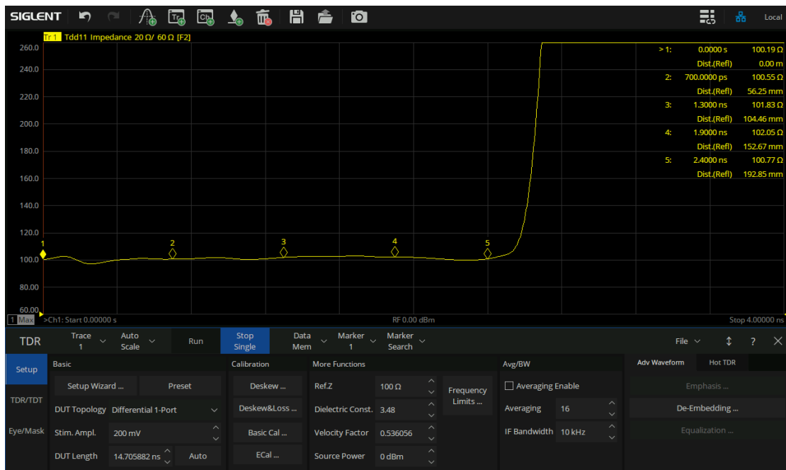
Figure 4-19 TDR test result of differential line
