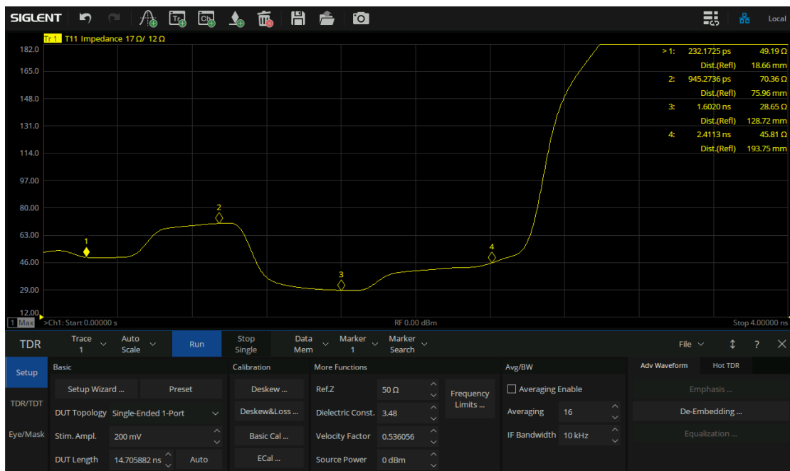
Figure 4-16 TDR test result of impedance transformation line
