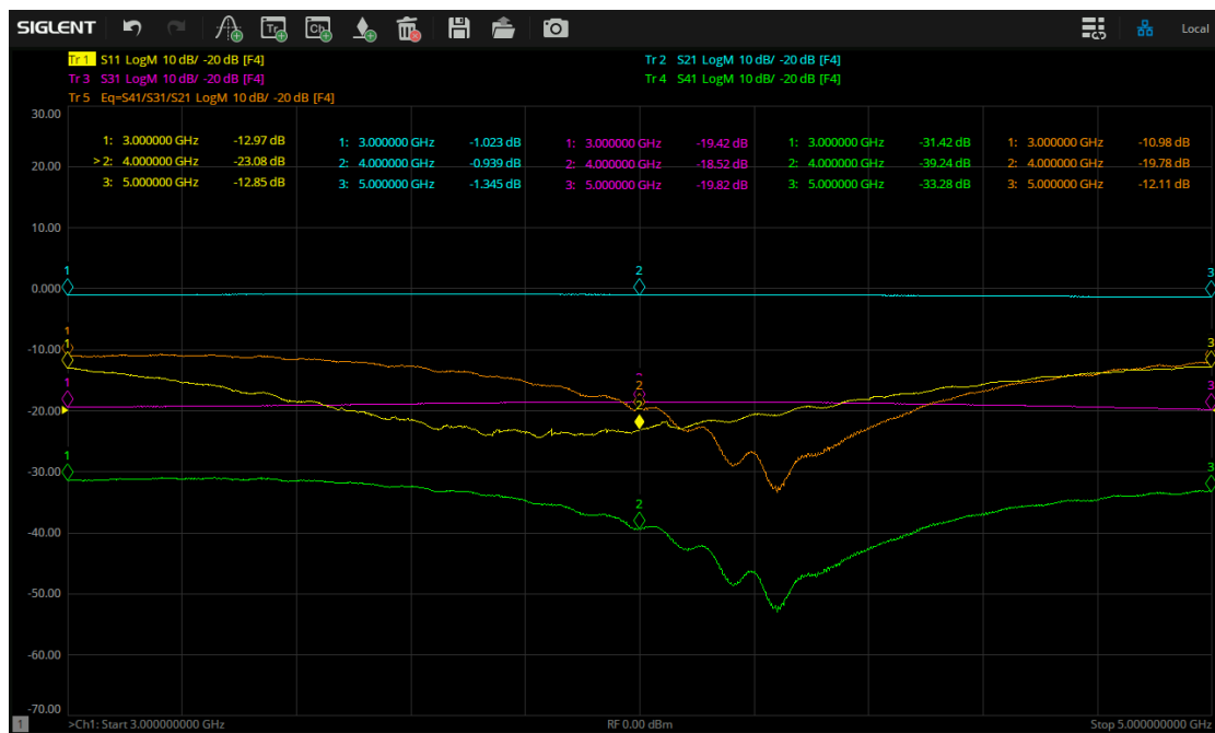
Figure 4-7 Test result of coupler
