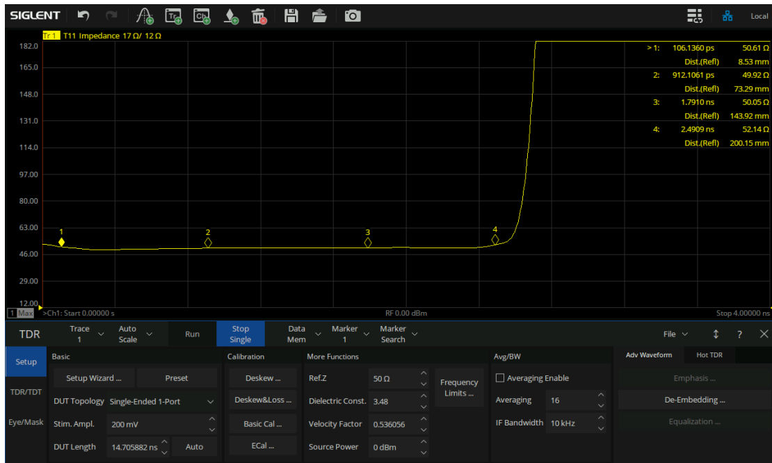
Figure 4-15 TDR test result of long through line
