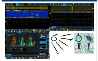
Difficult-to-find faults often result from the interaction between time and frequency signals. The R&S\*RTx-K18 spectrum analysis and spectrogram option quickly finds such errors. Parameters such as center frequency and resolution bandwidth can be easily adapted to the specific measurement task. The oscilloscope automatically selects the relevant time domain settings.
