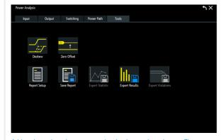
Add each result to the test report by simply pressing a button. The test report documents the setup and configuration. Define the level of detail in the report and customize the layout, for example by adding a company logo. The output format is PDF.
