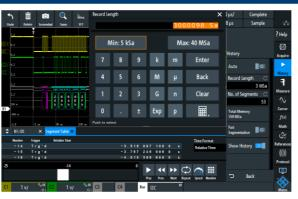
The history and segmented memory offer various user options, providing more flexibility for your applications. Automatic and manual memory configuration are available. In automatic mode, the instrument automatically defines the record length (number of waveform samples that are stored) and the number of history segments. In manual mode, you can set these parameters yourself.
