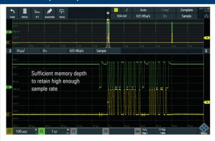
With sufficient memory, the oscilloscope can retain the maximum sample rate (and rated bandwidth) to accurately show the signal. With insufficient memory, the oscilloscope begins reducing the sample rate in order to capture more time. This can lead to insufficient sample rates to accurately show signals.
