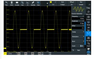
The R&S®RTx-B6 arbitrary waveform generator offers various user options, providing more flexibility for your applications. Besides different types of waveforms, the frequency, amplitude or offset can be set. For each waveform, you can configure the sweep and modulation type and add different burst signals.
