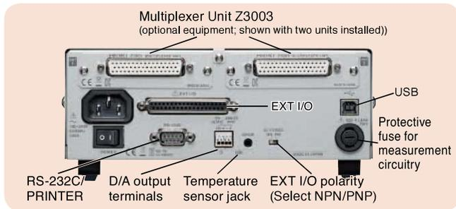
\*Multiplexer Units cannot be installed in the RM3545 or RM3545-01. The RM3545-01 has a GP-IB connector.
