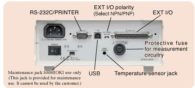
\*The RM3544 does not include EXT I/O or communication interfaces (RS-232C or USB). Select the RM3544-01 for these functions.
