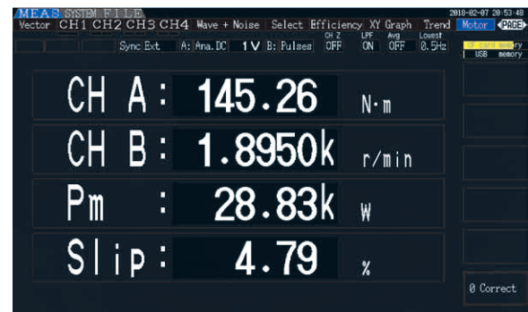
Motor analysis screen (Torque, rotation rate, motor power, slip)
