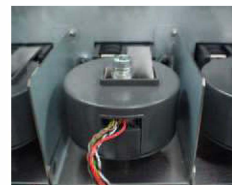
DCCT current sensor (in the PW3337)
