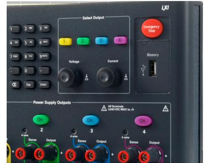
Figure 11. The N6705's front panel USB port.
