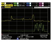
Figure 5. In Data Logger View, you can log data on multiple traces. Here, the current flowing out of output 1 and output 2 are captured over 30 seconds.
