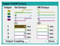
Figure 9. The Output On/Off Delays screen allows you to enter the delay times for each output. A graphical representation of the settings is shown
