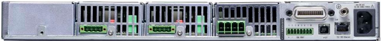
Figure 4. Rear panel (Picture shows 3 channels installed.)
