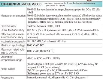
Cable length and mass: Main unit cable 1.5 m (4.92 ft), input section cable 1 m (3.28 ft), approx. 320 g (11.3 oz)
