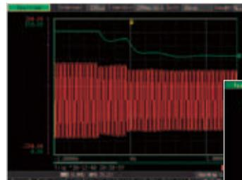
Record RMS values and instantaneous waveforms simultaneously.
