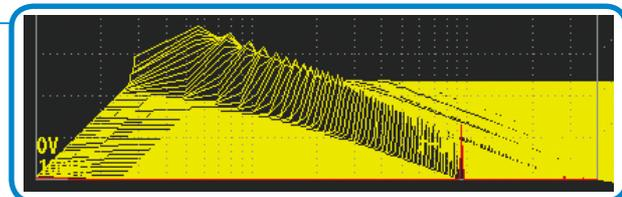
The MR8875 can also freeze the spectrum display on its screen during measurement. This function allows data to be observed without the inclusion of unneeded information on the screen or in the data. All calculation results can be output as CSV data, which can be loaded into a spreadsheet application such as Microsoft Excel and used to create a three-dimensional graph.
