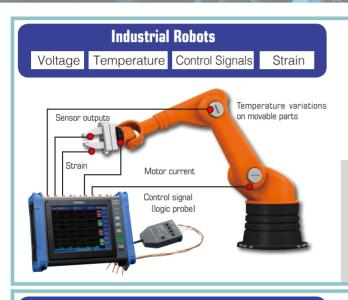
The plug-in module-based architecture means you can mix and record a variety of signals across multiple channels - ideal for verifying the operation of multi-axis robots.
