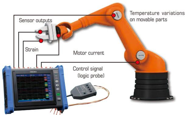
The plug-in module-based architecture means you can mix and record a variety of signals across multiple channels - ideal for verifying the operation of multi-axis robots.
