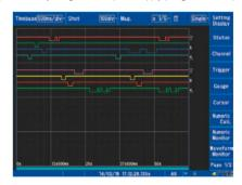
$\bullet \ \ \text{Multi-channel timing measurement using logic waveform measurement} \\$
