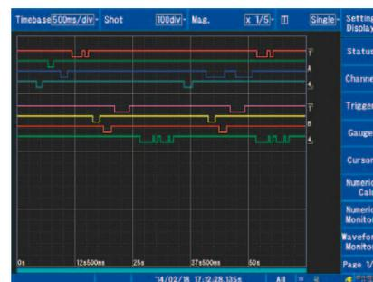
• Multi-channel timing measurement using logic waveform measurement
