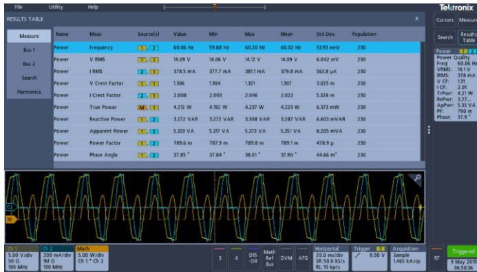
Power Quality measurement table. Automated power measurements enable quick and accurate analysis of common power parameters.
