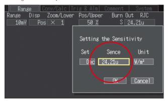
Simply enter the sensitivity of the heat flow sensor to complete the settings
