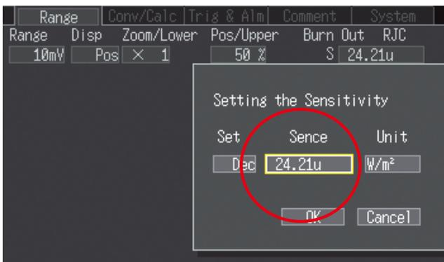
Simply enter the sensitivity of the heat flow sensor to complete the settings
