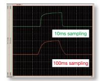
Measurement comparison of abrupt load change in waveform with 10 ms (upper trace) and 100 ms sampling
