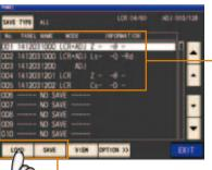
Save and load measurement conditions and compensation values.
