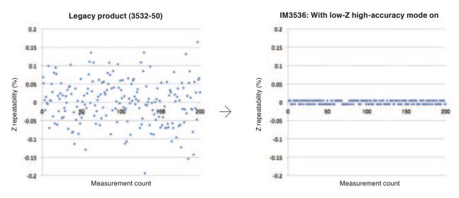
Graphs illustrate the results of measuring a resistance of 1 m $\Omega$  200 times under the following conditions:
