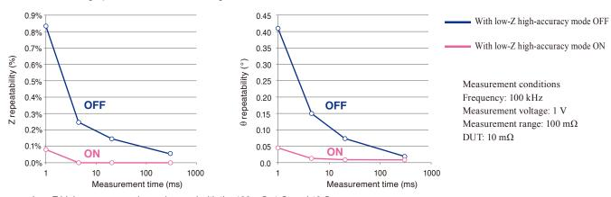
Low-Z high-accuracy mode can be used with the 100 m $\Omega$ , 1  $\Omega$ , and 10  $\Omega$  ranges. This mode is especially effective when performing low-inductance L measurement of power supplies and ESR measurement of aluminum electrolytic capacitors.
