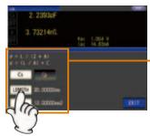
Enter the following parameters: \_ Conductor length (LENGTH) Conductor cross-sectional area (AREA)
