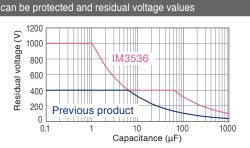
Relationship between the capacitance from which LCR meters
