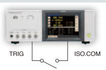
Select [External trigger] as the trigger setting and then control instrument operations such as measurement and saving of data from an external device such as a foot switch via the EXT. I/O terminal's TRIG signal.
