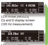
LCR mode [IM3523] Rs display screen (100 kHz measurement)
