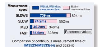
With continuous measurement under varying measurement conditions such as C-D + ESR measurement of capacitors, the total measurement time has been shortened significantly from the previous HIOKI model 3522-50. In addition to the reduction of the time required for individual measurements, the time required to change ranges such as a frequency range has been reduced significantly.
