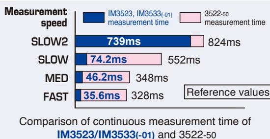
With continuous measurement under varying measurement conditions such as C-D + ESR measurement of capacitors, the total measurement time has been shortened significantly from the previous HIOKI model 3522-50. In addition to the reduction of the time required for individual measurements, the time required to change ranges such as a frequency range has been reduced significantly.
