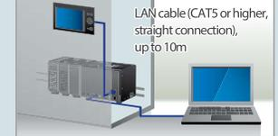
LAN cable (CAT5 or higher, straight connection), up to 10m
