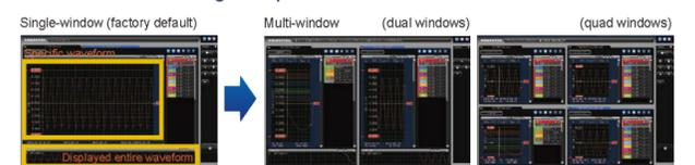
The complete measured waveform can be displayed on one screen. Displayed items in each window can be specified by the unit, the module, or channels. (ex. waveform measured in the each unit is displayed in the separate screens.)
