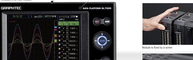
Attaching the high-definition display module with touch panel
