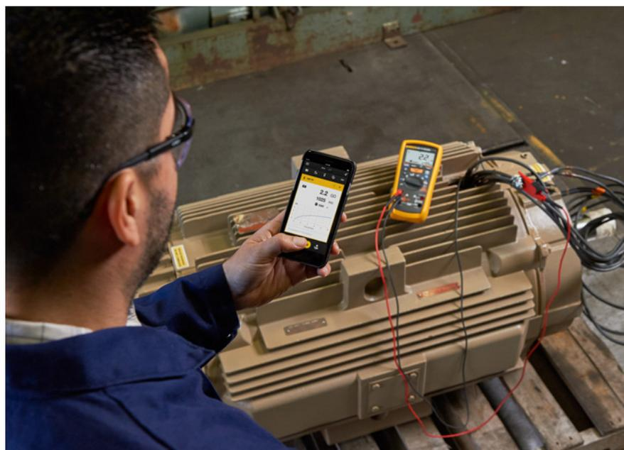
Store and share data using the Fluke 1587 FC with Fluke Connect Measurements App.
