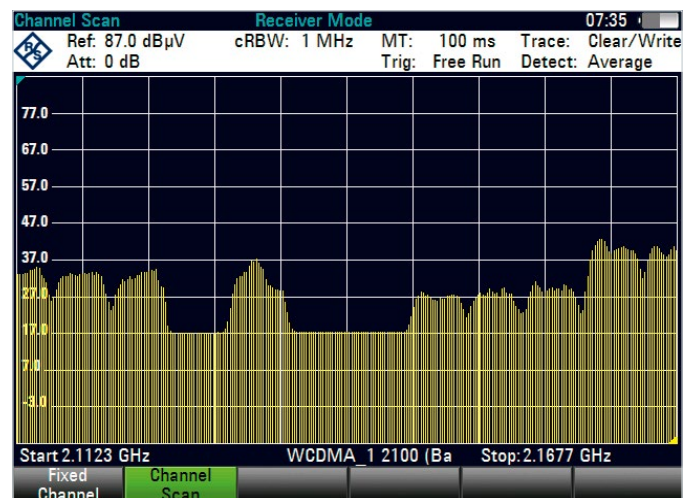
Channel scan of a 3GPP WCDMA frequency band.
