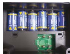
Compartiment piles / fusible
