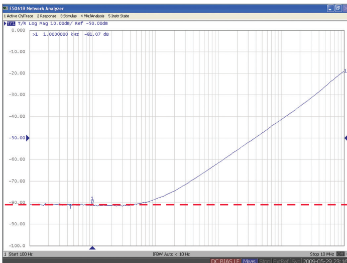
OP-amp PSRR measurement (100 Hz to 10 MHz)
