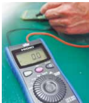
Test leads plug into the rear
