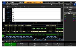
Figure 16. RS232 decode and trigger.
