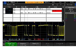
Figure 17. CAN-FD decode and trigger.
