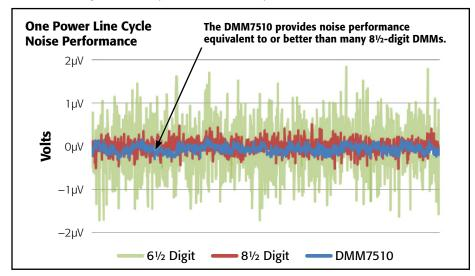
Comparison of the Model DMM7510's 1V DC noise performance with that of typical 6½- and 8½-digit multimeters. All data was taken at 1 NPLC with a low thermal short applied to the input.
