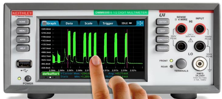
Analyze complex waveforms with the touchscreen display.
