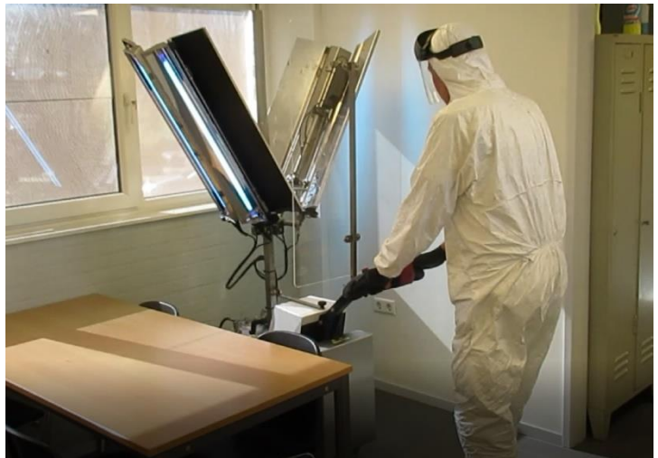
Fig. 1 : DIS-UV-GI disinfecting; flaps are open
