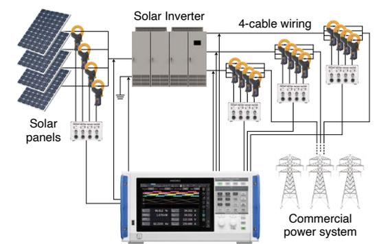
In large-scale solar power systems like megasolar installations, extremely large currents on the order of 1000 A to 3000 A branch out and flow through two to four wires. Current values of each wire measured with the CT6840A series sensors can be added for the total current value using the box-type CT9557 sensor unit. The total current value will be output as one signal to allow evaluation of PCS efficiency.
