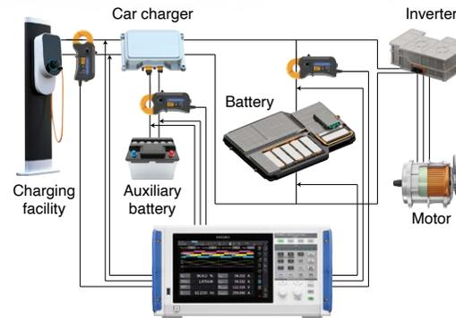
The "clamping" nature of the CT6840A series allows current measurement in an operating vehicle without requiring cables to be cut. When used in combination with a Hioki Power Analyzer, it can accurately perform current and power calculations for system batteries during charging and discharging as required for fuel efficiency measurements under the WLTP international standard.
