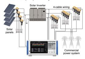
In large-scale solar power systems like megasolar installations, extremely large currents on the order of 1000 A to 3000 A branch out and flow through two to four wires. Current values of each wire measured with the CT6840A series sensors can be added for the total current value using the box-type CT9557 sensor unit. The total current value will be output as one signal to allow evaluation of PCS efficiency.
