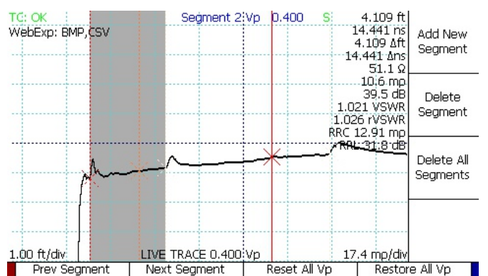
Figure 4: Multisegment cable with first segment VoP of 0.400.
