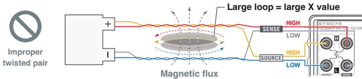
Loops increase the effects of induction flux caused by eddy currents, mutual interference, and peripheral equipment.
