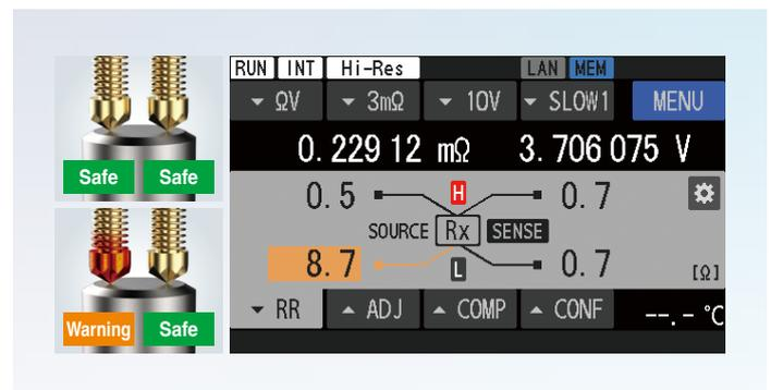
Monitoring route resistance and displaying a warning before a measurement error occurs
