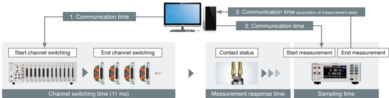
$$\text{Cycle time} = (\text{Communication time} + \text{Channel switching time} + \text{Measurement response time} + \text{Sampling time}) \times \text{Number of channels}$$
