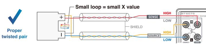
A more robust system can be attained by routing wires so as to minimize X values.
