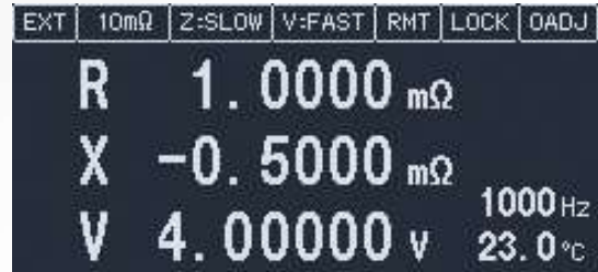
Measure 4-V Li-ion battery cells at an accuracy of \pm 190 \mu\text{V}
