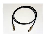
The N1412A/B/C Triaxial cable is suitable for low current applications down to the sub-fA level. It supports a maximum voltage/current of 500 V/1 A DC.
