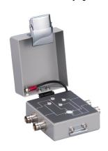
This test fixture has four triaxial connectors, allowing it to make two 2-wire connections or 4-wire connections. The N1295A test fixture supports up to 42 V and 1.05 A DC. It is compatible with the B2901A/02A/11A/12A and B2961A/62A.
