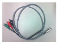
Triax cable terminated with a male triax connector on one end and three alligator clips on the other. It supports up to 200 V and 1A DC.
