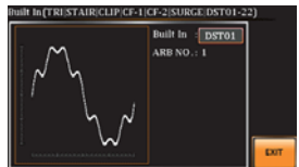
Fourier Series Synthesized Waveform
