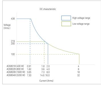
AC6800B steady-state AC output characteristic
