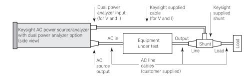
Figure 1. Test configuration of efficiency measurement using an Keysight AC source with the 020 dual power analyzer option.
