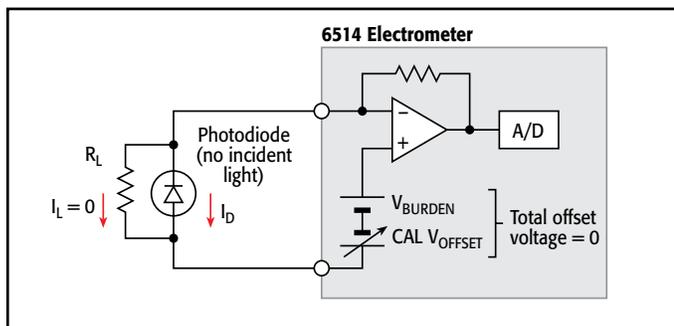
Figure 2. Dark Current Measurement with Burden Voltage Corrected
