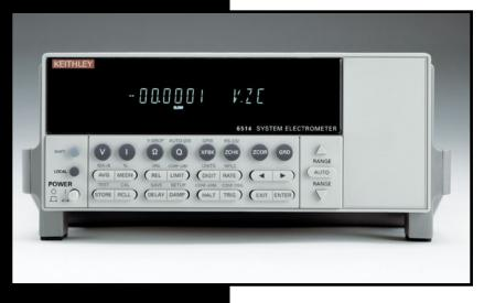
The Model 6514 Electrometer combines flexible interfacing capabilities with current sensitivity, charge measurement capabilities, resolution, and speed that are equal or superior to our earlier electrometers. The Model 6514's built-in IEEE-488, RS-232, and digital I/O interfaces make it simple to configure fully automated, high speed systems for low-level testing.
