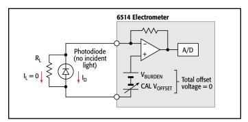
Figure 2. Dark Current Measurement with Burden Voltage Corrected
