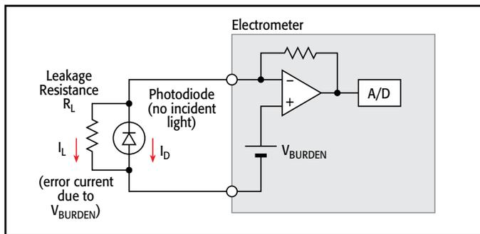
Figure 1. Dark Current Measurement with Burden Voltage Uncorrected
