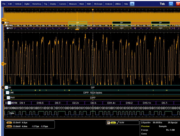
USB 3.0 bus display showing multiple layers simultaneously
