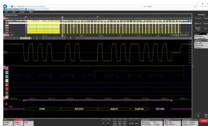
Figure 31: e*Scope provides simple remote viewing and control using common web browsers.
