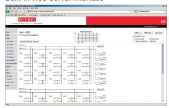
Configure your switch channels and measurement functions. Configure the DMM to make your measurements at the desired speed, resolution, etc. and assign them to the desired channels.
