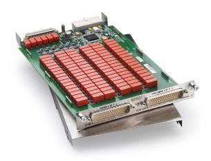
The 3730 is a two-pole, 6 row by 16 column matrix card. It can connect up to six differential instrument channels to any combination of 16 DUTs (devices under test). Any row can be connected to the Series 3700A mainframe backplane by using the analog backplane connection relays. This allows for easy matrix column expansion. A matrix of up to 6 rows by 96 columns can be supported within a single 3706A mainframe (with six 3730 cards).
