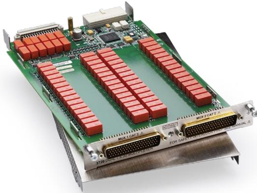
The 3720 offers two independent banks of 1x30 two-pole multiplexers. It is ideal for general purpose switching, including temperature measurements. The two banks can automatically be connected to the Series 3700A mainframe backplane and optional DMM through the analog backplane connection relays. This connection allows the mainframe to reconfigure the card to a single 1x60 two-pole multiplexer or to enable card-to-card expansion for even larger configurations.
