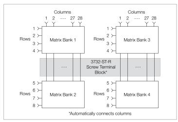
Dual 8×28 (1-wire) or single 8×28 (2-wire) matrix configuration using one 3732-ST-R screw terminal block
