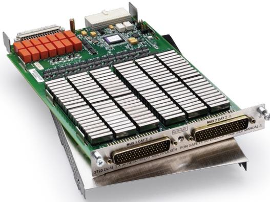
The 3723 offers two independent banks of high speed 1x30 two-pole multiplexers that are ideal for high speed scanning applications. The two banks can automatically be connected to the Series 3700A mainframe backplane and optional DMM through the analog backplane connection relays. This connection allows the mainframe to reconfigure the 3723 as a single 1x60 two-pole multiplexer or as a single 1x120 single-pole multiplexer. It also enables card-to-card expansion for even larger configurations.
