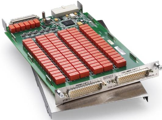
The 3730 is a two-pole, 6 row by 16 column matrix card. It can connect up to six differential instrument channels to any combination of 16 DUTs (devices under test). Any row can be connected to the Series 3700A mainframe backplane by using the analog backplane connection relays. This allows for easy matrix column expansion. A matrix of up to 6 rows by 96 columns can be supported within a single 3706A mainframe (with six 3730 cards).
