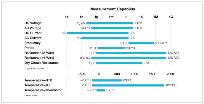
Measurement capabilities of the high performance multimeter
