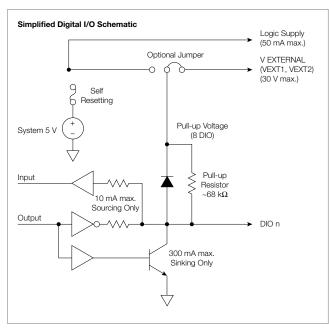
Figure 2. Simplified I/O schematic
