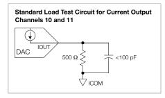
Figure 4. Standard load test circuits
