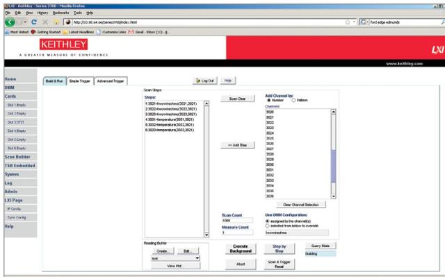
2. Build and run your automated scan list. The toolkit makes it easy to build and execute an automated sequence of channel-open and channel-close commands and triggered multimeter measurements.
