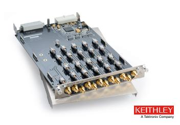
The 3761 provides quality low-current switching at an affordable price. The offset current error generated is specified <1pA, with typical performance at <30fA. When used with a voltage source and an electrometer or picoammeter, this card can easily automate insulation resistance tests, reverse leakage tests on semiconductor junctions, or gate leakage tests on FETs.
