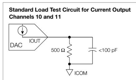
Figure 4. Standard load test circuits
