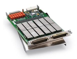
The 3723 offers two independent banks of high speed 1×30 two-pole multiplexers that are ideal for high speed scanning applications. The two banks can automatically be connected to the Series 3700A mainframe backplane and optional DMM through the analog backplane connection relays. This connection allows the mainframe to reconfigure the 3723 as a single 1×60 two-pole multiplexer or as a single 1×120 single-pole multiplexer. It also enables card-to-card expansion for even larger configurations.
