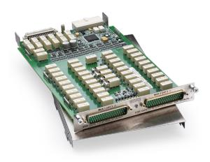
The 3721 offers two independent banks of 1×20 two-pole multiplexers that are ideal for general purpose switching, including temperature measurements. The two banks can automatically be connected to the Series 3700A mainframe backplane and optional DMM through the analog backplane connection relays. This connection allows the mainframe to reconfigure the 3721 as a single 1×40 two-pole multiplexer or to enable card-to-card expansion for even larger configurations.
