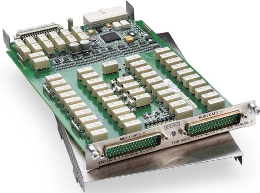
The 3721 offers two independent banks of 1x20 two-pole multiplexers that are ideal for general purpose switching, including temperature measurements. The two banks can automatically be connected to the Series 3700A mainframe backplane and optional DMM through the analog backplane connection relays. This connection allows the mainframe to reconfigure the 3721 as a single 1x40 two-pole multiplexer or to enable card-to-card expansion for even larger configurations.
