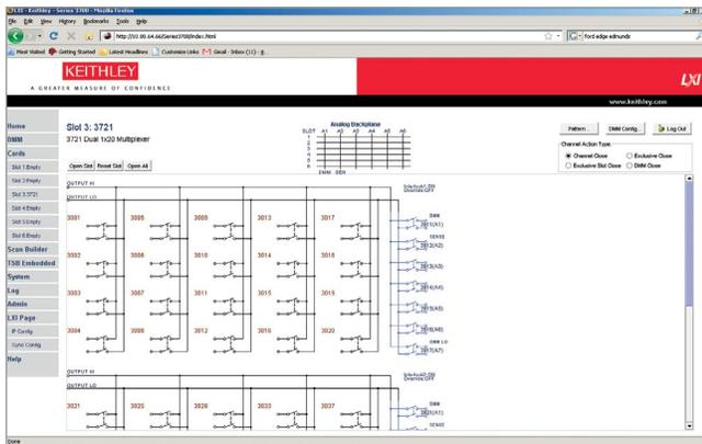
1. Configure your switch channels and measurement functions. Configure the DMM to make your measurements at the desired speed, resolution, etc. and assign them to the desired channels.
