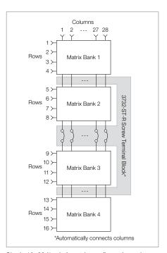
Single 16×28 (1-wire) matrix configuration using one 3732-ST-R screw terminal block
