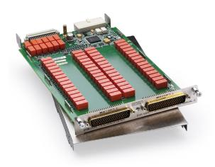
The 3720 offers two independent banks of 1×30 two-pole multiplexers. It is ideal for general purpose switching, including temperature measurements. The two banks can automatically be connected to the Series 3700A mainframe backplane and optional DMM through the analog backplane connection relays. This connection allows the mainframe to reconfigure the card to a single 1×60 two-pole multiplexer or to enable card-to-card expansion for even larger configurations.
