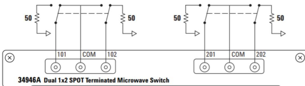
Figure 15. 34946A dual 1x2 SPDT terminated microwave switch
